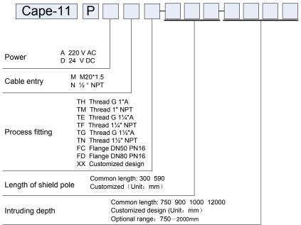
Note: The number of intruding depth and length of shield poles are fixed at three and four digits respectively, If the number of real depth or length is less than the required fix digits, zero should be added in front of its number. For example: The length of shield pole is 90mm, expressed as "090"; the intruding depth of 750mm, expressed as "0750".
