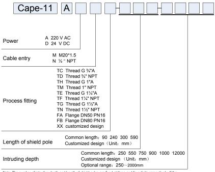
Note: The number of intruding depth and length of shield poles are fixed at three and four digits respectively, If the number of real depth or length is less than the required fix digits, zero should be added in front of its number. For example: The length of shield pole is 90mm, expressed as "090"; the intruding depth of 750mm, expressed as "0750".
