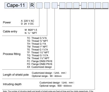
Note: The number of intruding depth and length of shield poles are tixed at three and four digits respectively, if the number of real depth or length is less than the required fix digits, zero should be added in front of its number. For example: The length of shield pole is 90mm, expressed as "090"; the intruding depth of 750mm, expressed as "0750".
