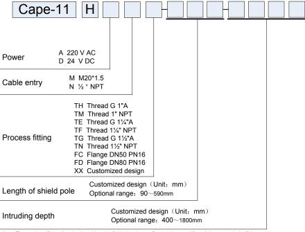
Note: The number of intruding depth and length of shield poles are fixed at three and four digits respectively, If the number of real depth or length is less than the required fix digits, zero should be added in front of its number. For example: The length of shield pole is 90mm, expressed as "090"; the intruding depth of 750mm, expressed as "0750".
